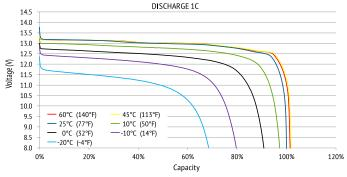
DISCHARGE VOLTAGE CHARACTERISTICS at VARIOUS TEMPERATURES
