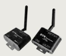
**Zigbee to USB converter & Zigbee to RS485** Zigbee to USB converter, DRF2618A, DTK Zigbee to RS485 converter, DRF2619A, TDK
