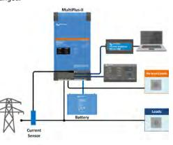
Standard mobile or off-grid application with external current sensor The 100A external current sensor extends the PowerControl and PowerAssist function to 100A.
