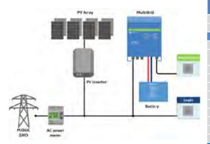
Grid parallel topology with PV inverter Similar to Hub 4-2 but in this topology the PV inverter will shut down in case of a power outage. Certain critical loads only are protected against a power outage.
